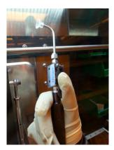
2. Use vacuum wand to load and unload substrate. Adjust the pressure of the glovebox with foot paddles if needed.
