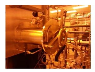
\*Turn on the pump. Loose the (counterclockwise) vacuum gate knob to pump down the loadlock and wait for the gauge reaches <-27 in.Hg and tighten (clockwise) the knob. Then turn the N2 valve to the right to fill up the loadlock and wait for the gauge to go back to 0.
