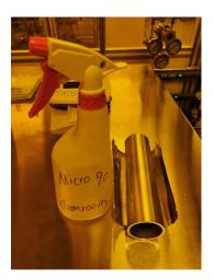
Spray a thin coat of Micro 90 2% solution onto the cold trap and use wipe to clean the liquid.
