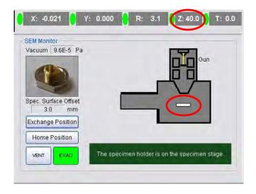
(6) A holder selection popup will appear. Select the correct the sample holder and put offset in if needed (offset value is how much taller from the sample surface to the top edge of the sample holder)
