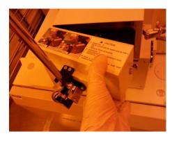
(5) Use the ROD to insert the sample stage into the main chamber. The stage icon should be in the main chamber and Z value is 40mm.
