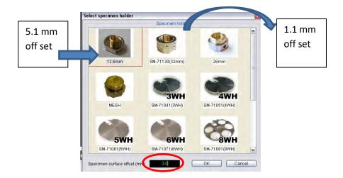
(7) Make sure the is green. Choose the WD (normal setting is 10 mm), click "OK" to have stage Z moved to the WD setting. Normal setting for Acceleration Voltage is at 15KV.
