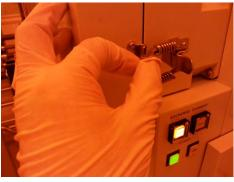
(3) Open the loadlock and push the sample holder onto the holding mechanism. Make sure the arrow side is on the top. Once the sample is secured, close the loadlock door and put the clamp back on. DO NOT PUSH on the ROD!!
