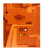
(4) Click "EVAC" to evacuate the loadlock chamber. It will take few minutes. Wait until the "EVAC" button on the loadlock side wall stop flashing.
