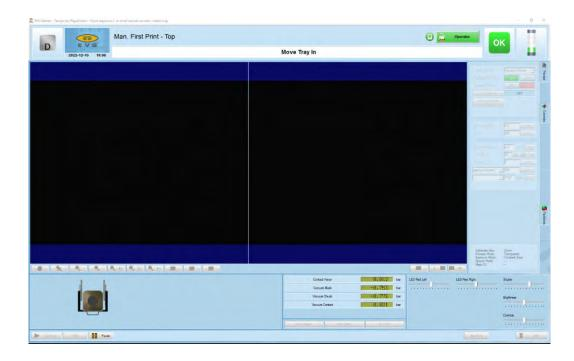
Align Substrate and Press "Continue". Only need to do the alignment step if alignment is needed. For flood exposure, press "Continue".
